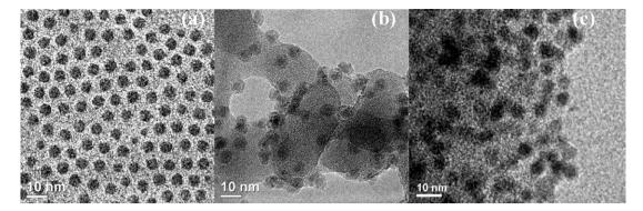
Fig. 1. TEM images of (a) colloidal Ni nanoparticles, (b) Ni/SiO<sub>2</sub> and (c) Ni/C.
