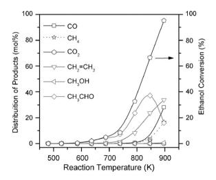
**Fig. 8.** Products distribution of steam reforming of ethanol. Reaction conditions: 0.120 g of catalyst (10 wt% Ni/SiO<sub>2</sub>); reactor fed with a mixture  $H_2O$ -ethanol (6:1 mol/mol, 2 mL  $h^{-1}$ ); helium was used as carrier gas.
