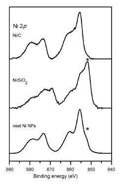
Fig. 2. Ni 2p core-level XP spectra of neat Ni NPs, and supported Ni NPs on silica and on activated carbon. The asterisks indicate Ni(0) component.
