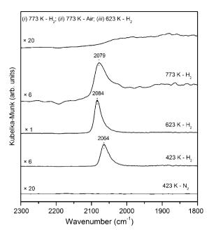
**Fig. 6.** DRIFT-spectra of CO adsorbed at room temperature on a Ni/SiO<sub>2</sub> sample treated at different temperatures (423, 623 and 773 K) and atmosphere (N<sub>2</sub>, H<sub>2</sub> or air). The upper curve was obtained after treating the sample at 773 K in H<sub>2</sub>, then in air at same temperature followed by a reduction at 623 K with H<sub>2</sub>. Note that each curve has a different intensity scale.
