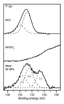
Fig. 4. P 2p core-level XP spectra of neat Ni NPs, Ni/SiO<sub>2</sub> and Ni/C samples.
