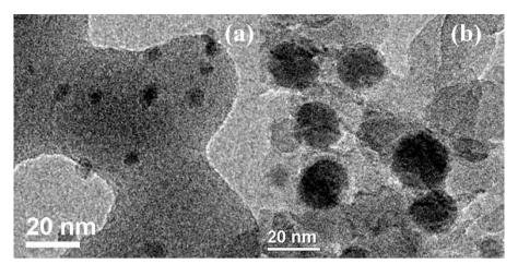
Fig. 7. TEM images of: (a) Ni/SiO<sub>2</sub> reduced at 623 K and (b) Ni/SiO<sub>2</sub> reduced at 773 K.
