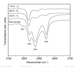
Fig. 5. DRIFT-spectra of Ni/SiO<sub>2</sub> fresh sample and after reduction at 423, 623 and 773 K. All spectra were taken at room temperature.
